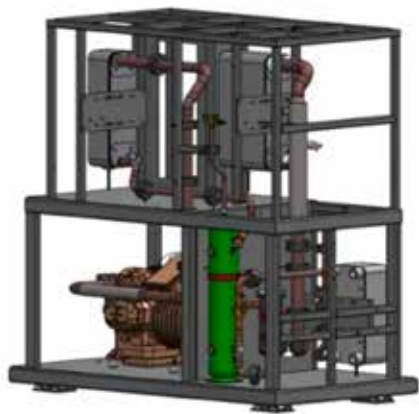
Developed within an extremely short span of time: new large heat pump delivering 200 kW thermal output and a flow temperature of up to 90 °C
